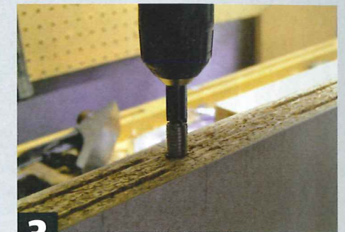
3 A special driver bit is available to drive the Invis fixings into the holes
