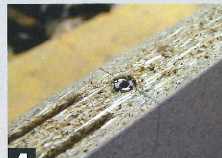
4 They should sit marginally below the surface, as shown
