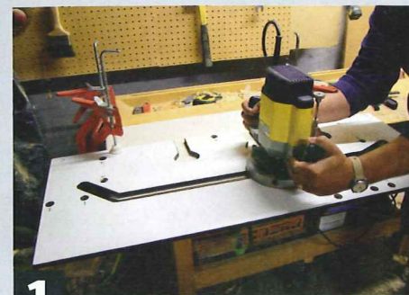
1 The worktop joint is cut in the normal manner, using a jig and router
