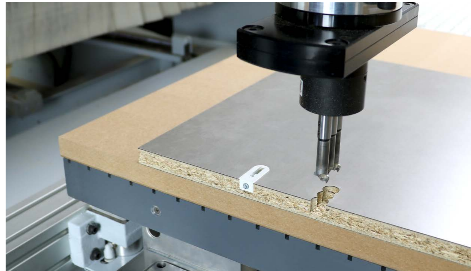
The connector pockets are machined by the multi-spindle head in one single step.
